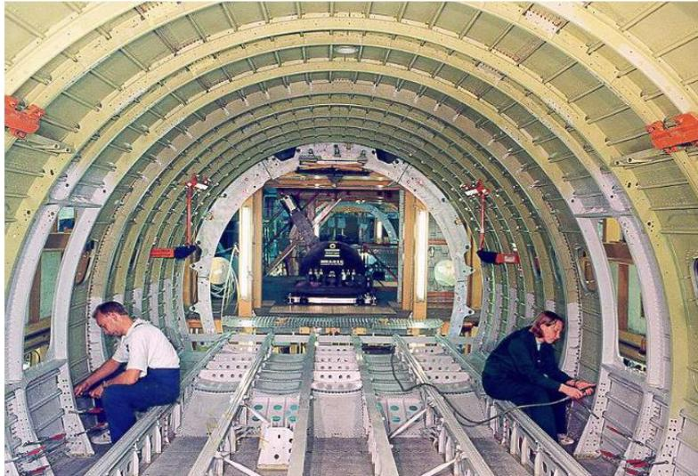
The structure of the fuselage of an aircraft.
